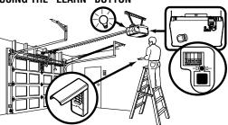
Press and release the "learn" button on motor unit. The learn indicator light will glow steadily for 30 seconds.
